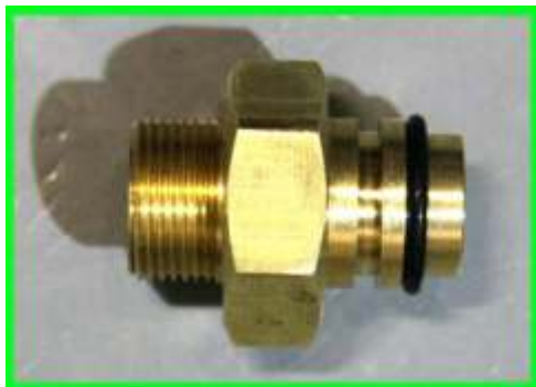
Fig. 4.5.2 – O-ring must fit against first shoulder, not in groove.
