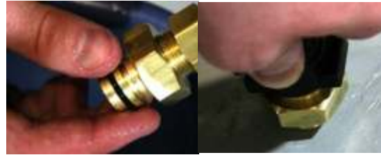
Fig. 4.5.3 – Wet o-ring to facilitate installation. Firmly press meter body over fitting to seat.
