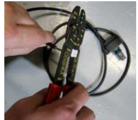
Fig. 4.10.6 – Cut off white connector if applicable.
