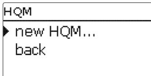
In the **HQM** menu, up to seven internal energy meterings energy meterings can be activated and adjusted. By selecting the menu item **new HQM...**, an new energy metering can be activated.
