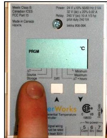
Fig. 7.1 – Changing display between Fahrenheit ( $^{\circ}F$ ) and Celsius ( $^{\circ}C$ )
