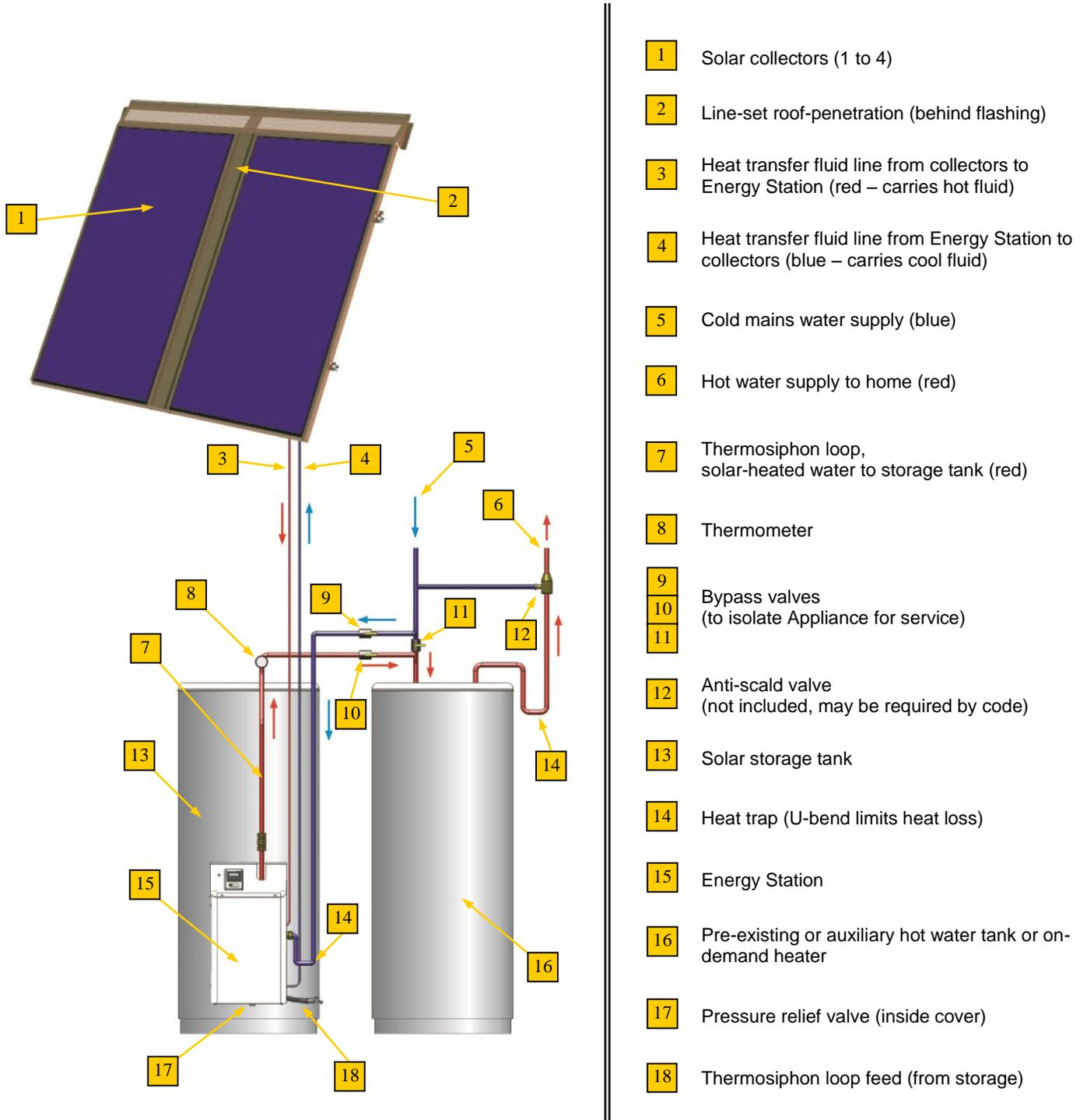
Fig.2.2 – EnerWorks Pre-Heat Solar Water Heating Appliance (with optional leaf-guard).
