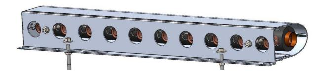
Fix, adjust and tighten the manifold with screw and nut.
