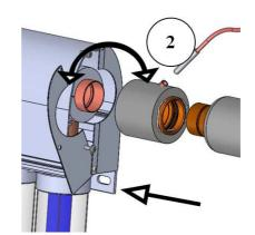
**Sensor pocket mounting:** Insert the sensor pocket into the thermometer pocket and connect it with the shrink hose. Shrink the shrink hose with a heating source or stick it with the added protective sheet.
