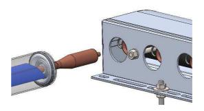
Now insert the tube into the manifold. Check the right position of the clips and the locking device by pulling slightly.
