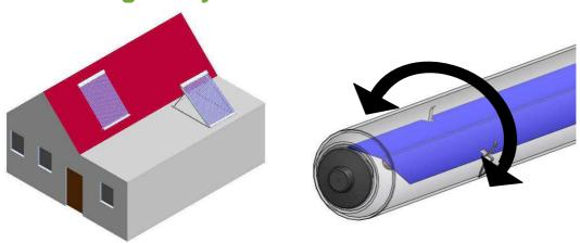
For a domestic water heating system, we recommend to adjust the absorber 45° to the sun. For a combination of domestic water heating and heating support, we recommend an angle of 60° to the sun.
