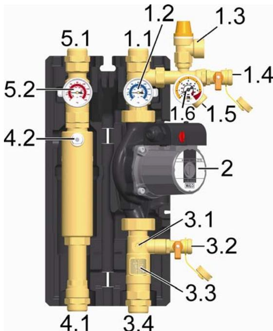
4. Close the drain valve [3.2] with the filling pump running and increase the system pressure, depending on the design of the system, to max. 5 bar. The pressure can be read on the pressure gauge. Close the fill valve [1.4] and switch off the pump of the flush and fill station.
