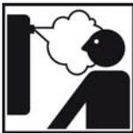
If the system pressure is too high, hot solar fluid will escape from the pressure relief valves and can result in scalding.
