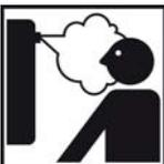
The valves and fittings may heat up to more than 212 °F (100 °C). During maintenance or decommissioning, the solar fluid may escape as vapor and result in scalding!
