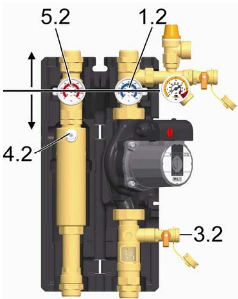
1. Gaskets below the ball valves: Perform partial draining as described in **6.1 Partial draining of the solar installation [specialist]**.
