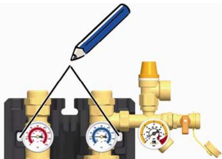
3. Copy the mounting holes next to the temperature gauges of the solar station to the mounting surface.
