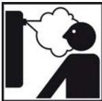
The escaping solar fluid can have a temperature of more than 212 °F (100 °C) and cause scaldings.
