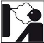
The valves and fittings may heat up to more than 212 °F (100 °C). During flushing, filling and venting, the solar fluid can escape as vapor and result in scalding.
