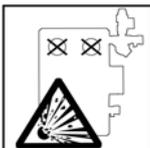
Closing both ball valves will disconnect the safety assembly from the heat exchanger. Heating the storage tank can result in the formation of high pressures, which may lead to material damage and personal injury!
