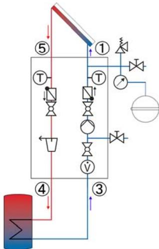
5. Connect the solar station to the system by means of pipes
